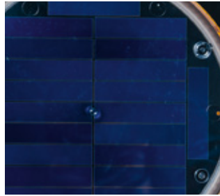
Solar Modules High-efficiency cells. Maximum Power Point Tracking (MPPT) for optimal energy collection.
