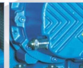
Immediate view of oil level
